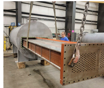
Dual-Circuit ES Cooler Bundle Insertion
