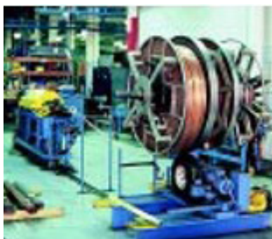
Use of rolled coil tubing supports the flexibility inherent in OFT manufacturing. Special straightening equipment and unique burr-free cutting process for superior rolled joints.
